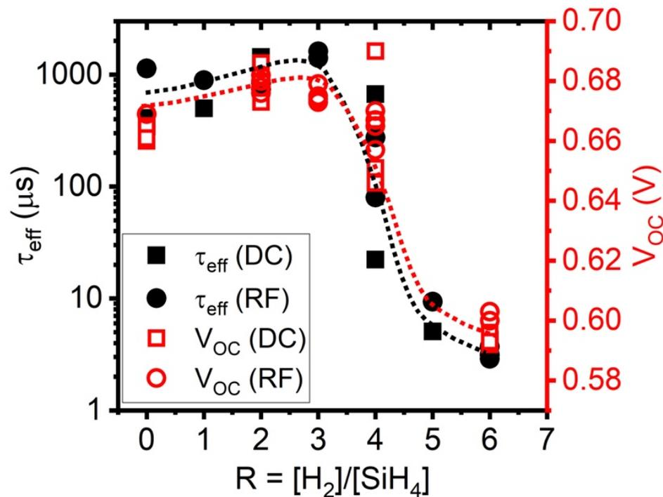
Effective lifetime (black) and  $V_{\text{OC}}$  (red) for a-Si/c-Si HJ solar cells deposited by RF or DC plasma for different H dilution ratios  $R_{\text{H}}$ .
