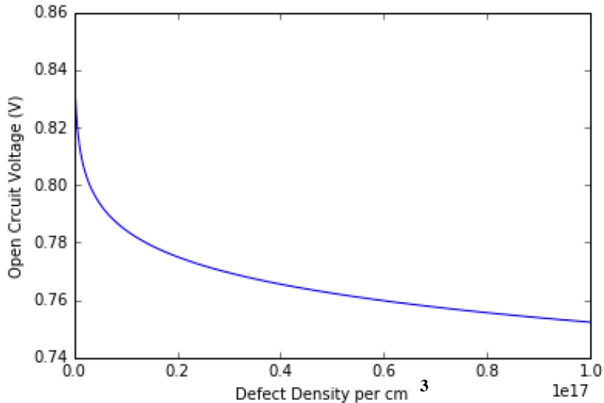
This curve translates the defect density  $n_{\text{def}}(t)$  into a time dependent Voc degradation
